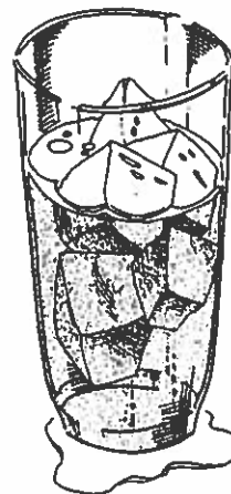
A common example of moisture condensation is the glass of ice water that "sweats."
